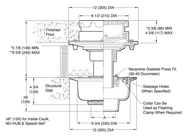
NOTE: \*Add 1/4"(6) for Nickel Bronze or Polished Bronze Top. \*\* If greater dimension than shown from lower flange to top is required specify a longer nipple. A (Pipe Size) = 02(50), 03(75), 04(100)
